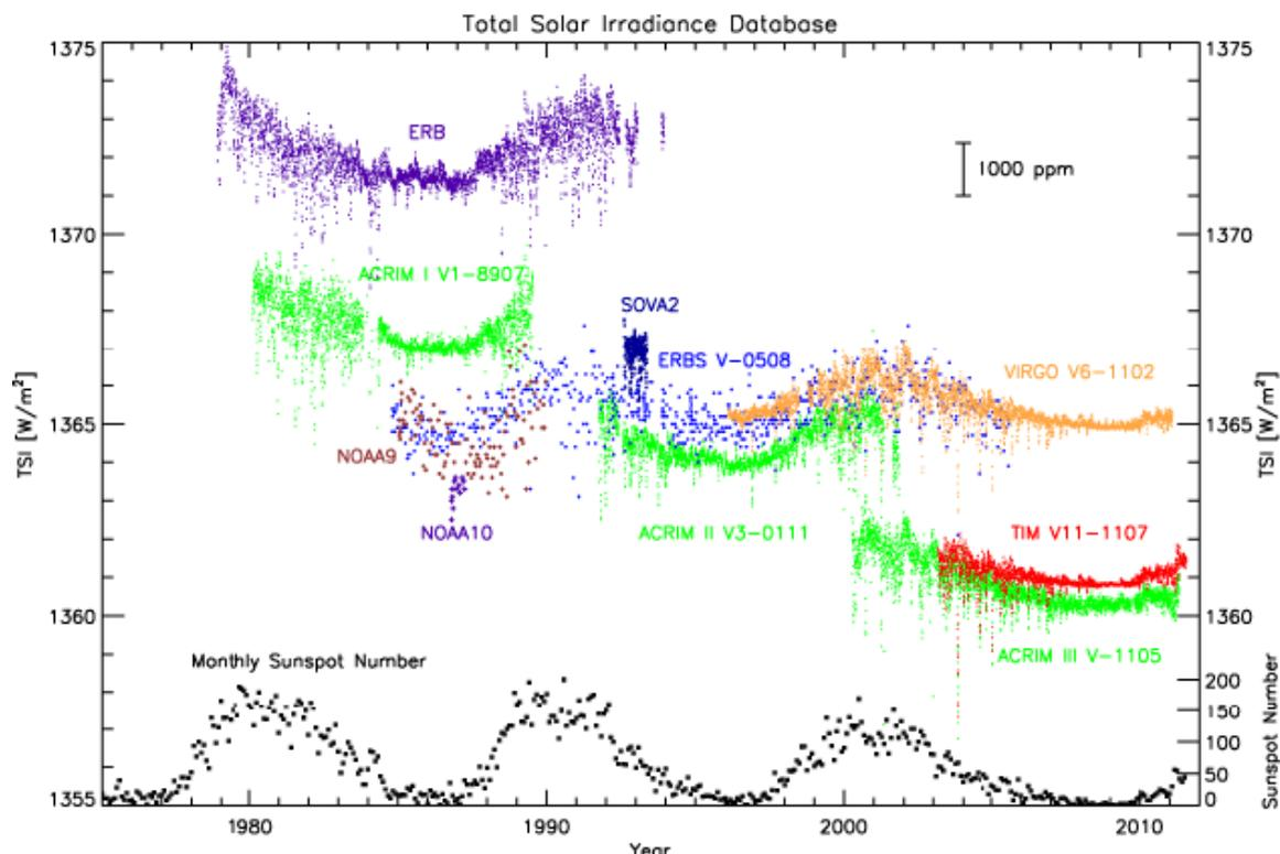
FIGURE C.1 The 33-year TSI record is the result of measurements made by several instruments. Measurement overlap helps correct for the majority of the differences between instruments, but instrument calibration is needed to provide the required accuracies and stabilities in this solar climate data record for reliable climate studies. SOURCE: Courtesy of G. Kopp, University of Colorado.
